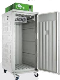
The Koala Green refrigerated containers are powered by a LiFePO4 battery, making them completely autonomous and independent from a vehicle. The removable battery can be recharged by connecting the Koala Green to the mains power(230V) or with an external charger after removing it from the refrigeration unit.
