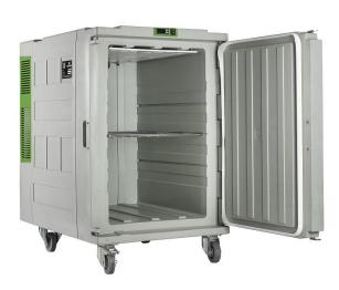
The Koala Green refrigerated containers are powered by a LiFePO4 battery, making them completely autonomous and independent from a vehicle. The removable battery can be recharged by connecting the Koala Green to the mains power(230V) or with an external charger after removing it from the refrigeration unit.
