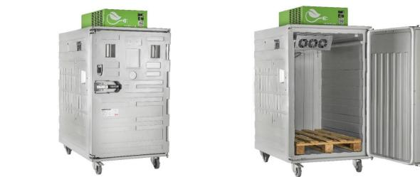
Koala Green refrigerated containers are powered by a LiFePO4 battery, making them completely autonomous and independent of a vehicle. The removable battery can be recharged by connecting the Koala Green to the mains power (230V) or with the external charger after removing it from the refrigeration unit.
