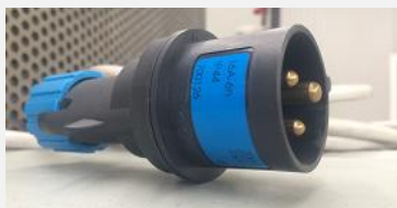
Picture 3 - IEC309 blue plug (2 poles + 230V 16A ground) for connection to 230Vvac 50-Hz power supply
