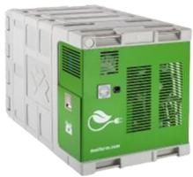
The Koala Green refrigerated containers are powered by a LiFePO4 battery, making them completely autonomous and independent from a vehicle. The removable battery can be recharged by connecting the Koala Green to the mains power(230V) or with an external charger after removing it from the refrigeration unit.
